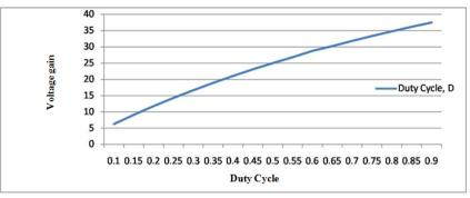
Fig. 5. Voltage gain of the proposed circuit throughout the duty cycle 0.1 to 0.9
