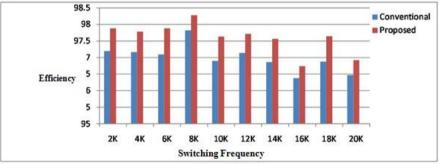
Fig. 4(a). Comparison of conventional and proposed circuit, Efficiency verses switching frequency
